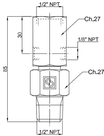
**TABLE 26: General characteristics of rupture discs 3070**
